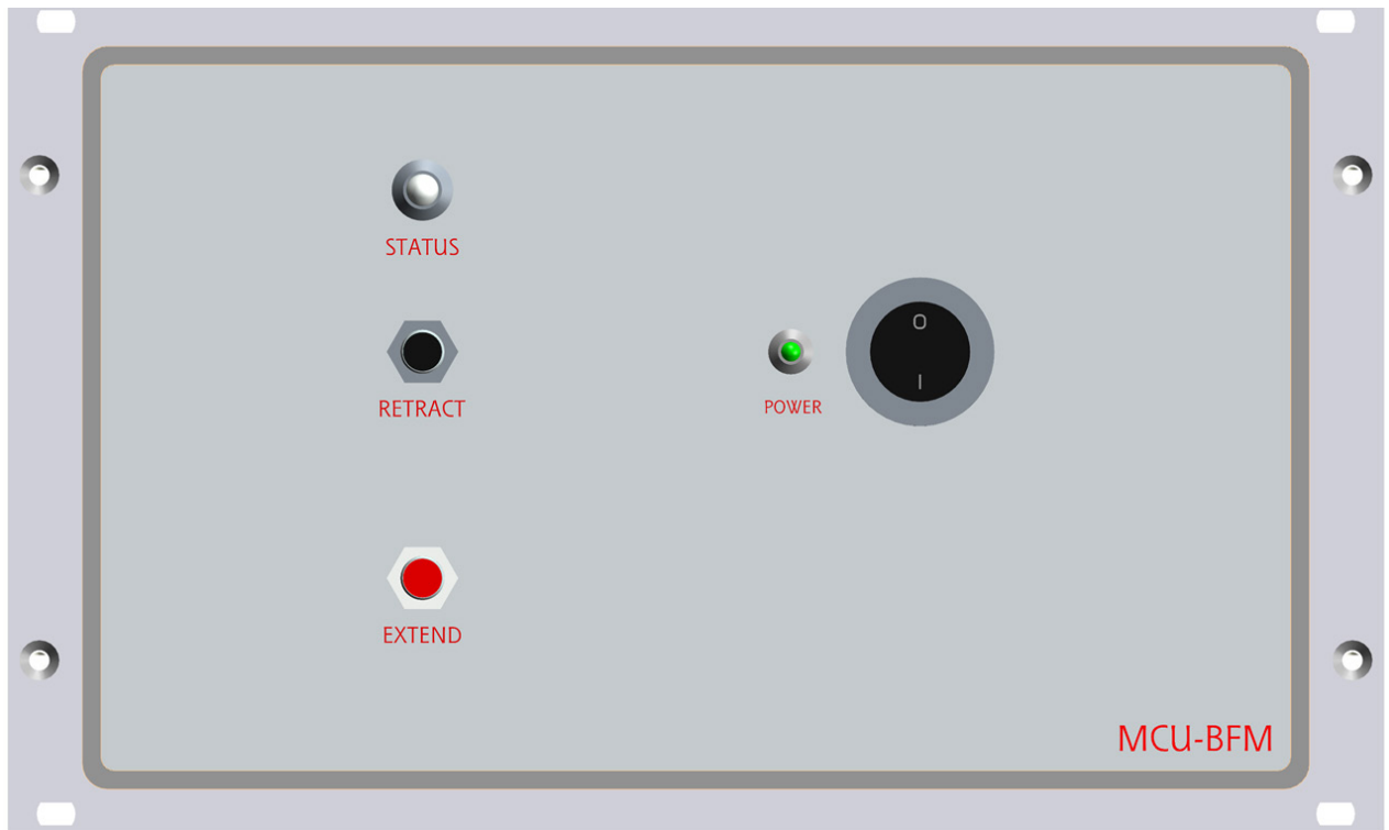
Fig. 3-4 Motor control unit (BFM) front panel with a Status LED, black push button for Park/Retract, red push button for Measure/Extend, a motor power switch, and a small Power LED. The Beam Flux Monitor should only be used with the original accessories supplied; these are listed in Table 2 below.
