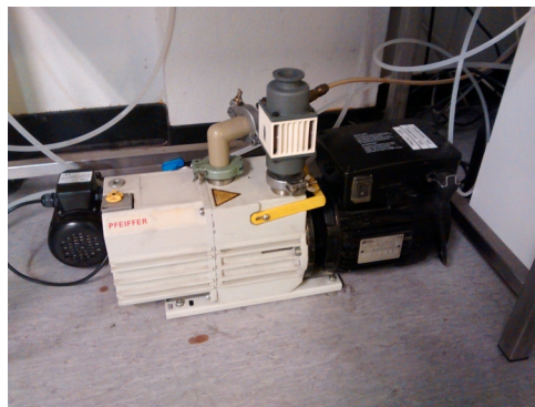
Illustration 4: Vacuum pump used by the mask aligner.
