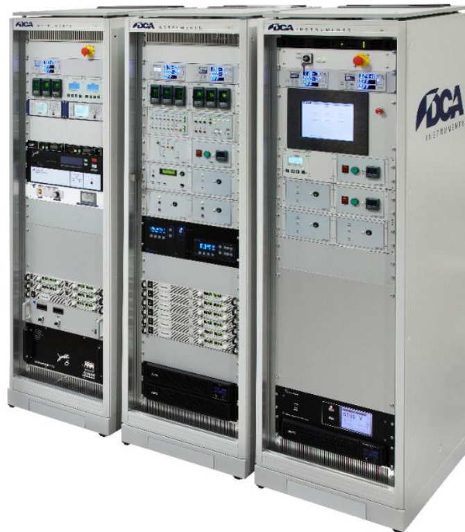
Fig. 6-1 The electronic racks house the peripherals, PC-based computer, power distribution panels, and EPO for the entire UHV deposition system.
