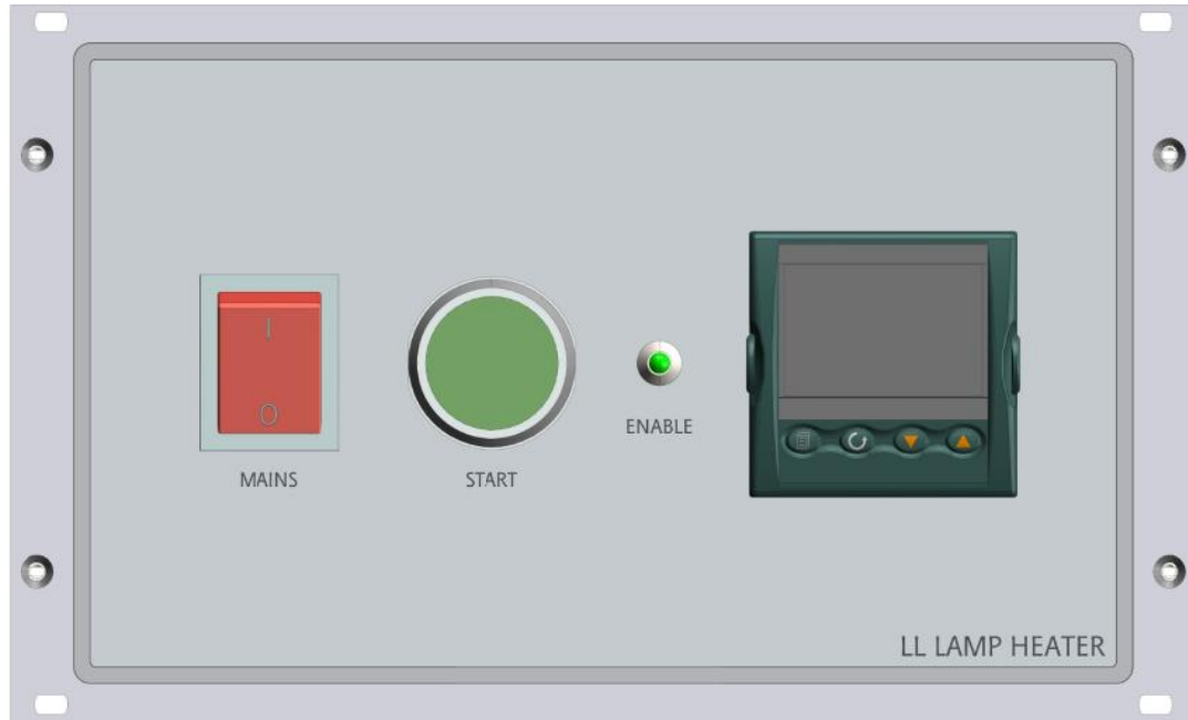
Fig. 5-6 Load lock lamp heater controller of the IR lamp heater allows the user to set the temperature (max. 200 °C) and duration.
