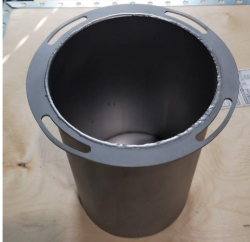
Fig. 4-1 Protective transfer tube with slots to secure the manipulator mounting flange.
