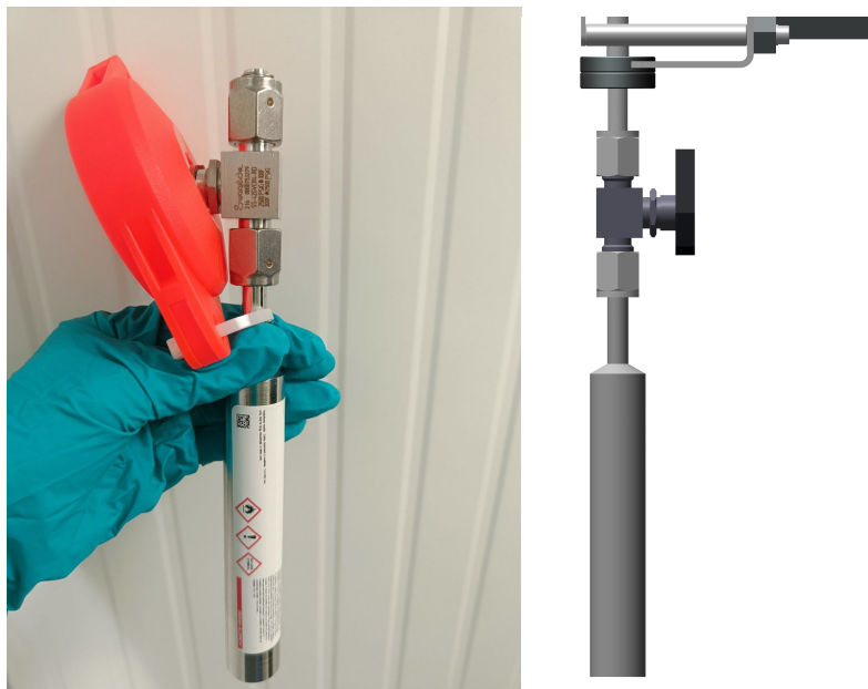
Fig. 6-1 Left: example of the ampule/source tank (left) with a sealed manual valve and VCR cap. Right: shows how the tank is mounted to the MOPI system.
